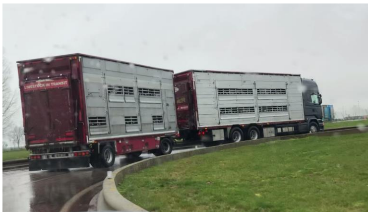
Slats on both sides of the trucks are open, resulting in wind and rain coming into the truck
