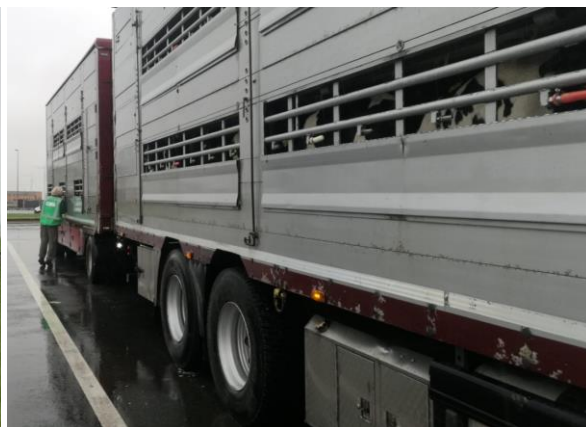
Slats on both sides of the trucks are open, resulting in wind and rain coming into the truck
